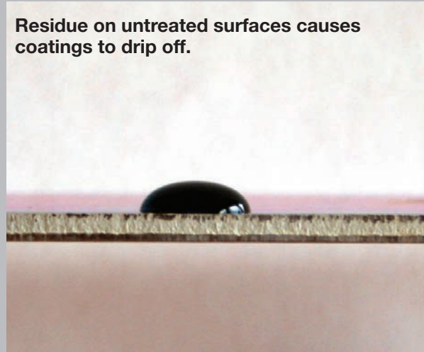
Plasma precision cleaning: A prerequisite for perfect adhesion
